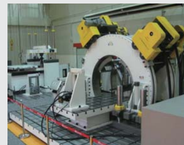
레일체결장치 다축 피로시험장비 Multi-Axial Fatigue Testing System for Rail Fastening System & Components
